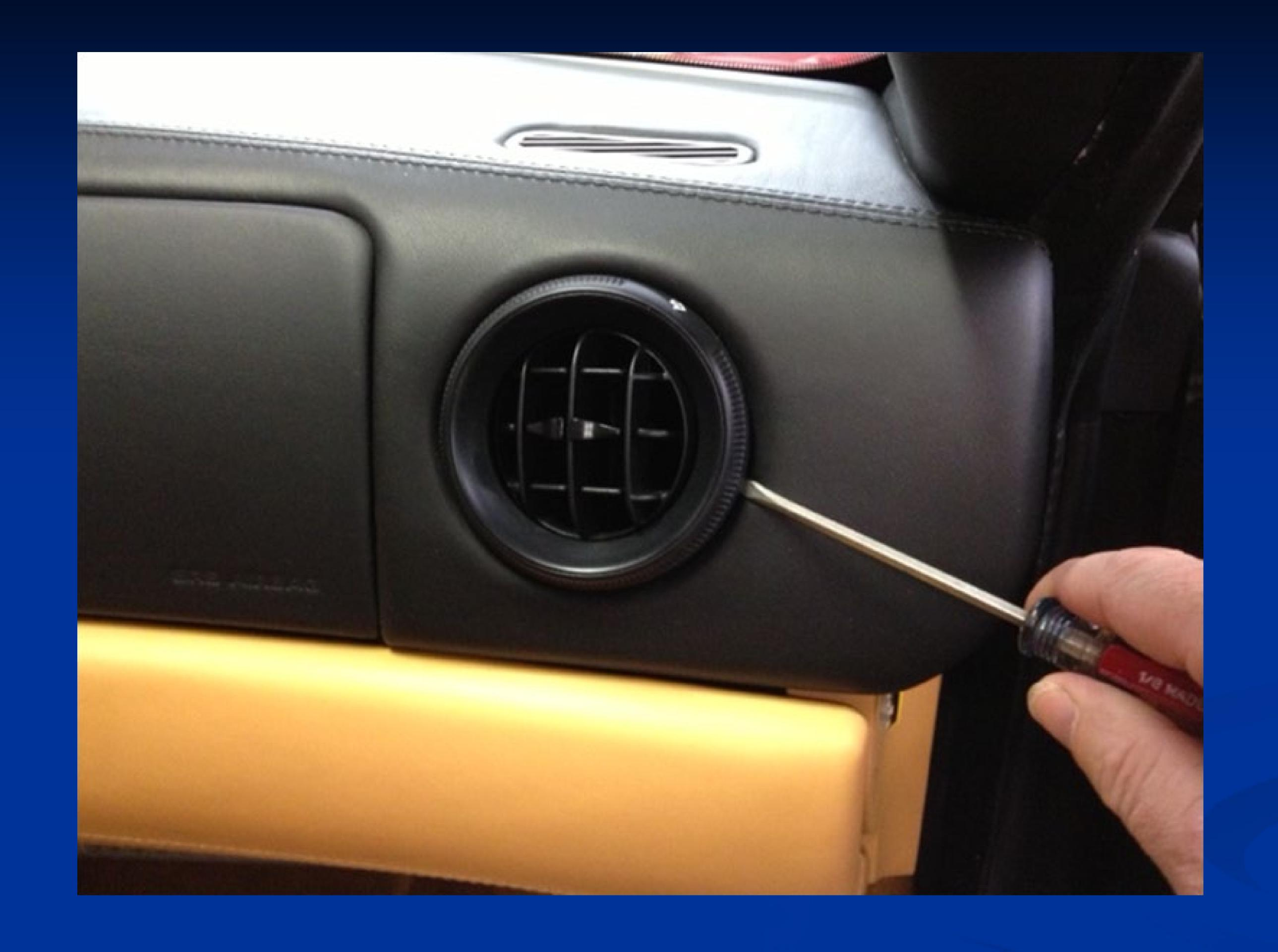
Gently twist the screwdriver either way and you will feel the vent ring start to pop off, move your screwdriver around the outer edge of the ring in 4-5 places each time gently insert the screwdriver in the gap and twist. The ring will pop right off into your hand. The next pic shows the ring completely unsnapped from the inner vent.
