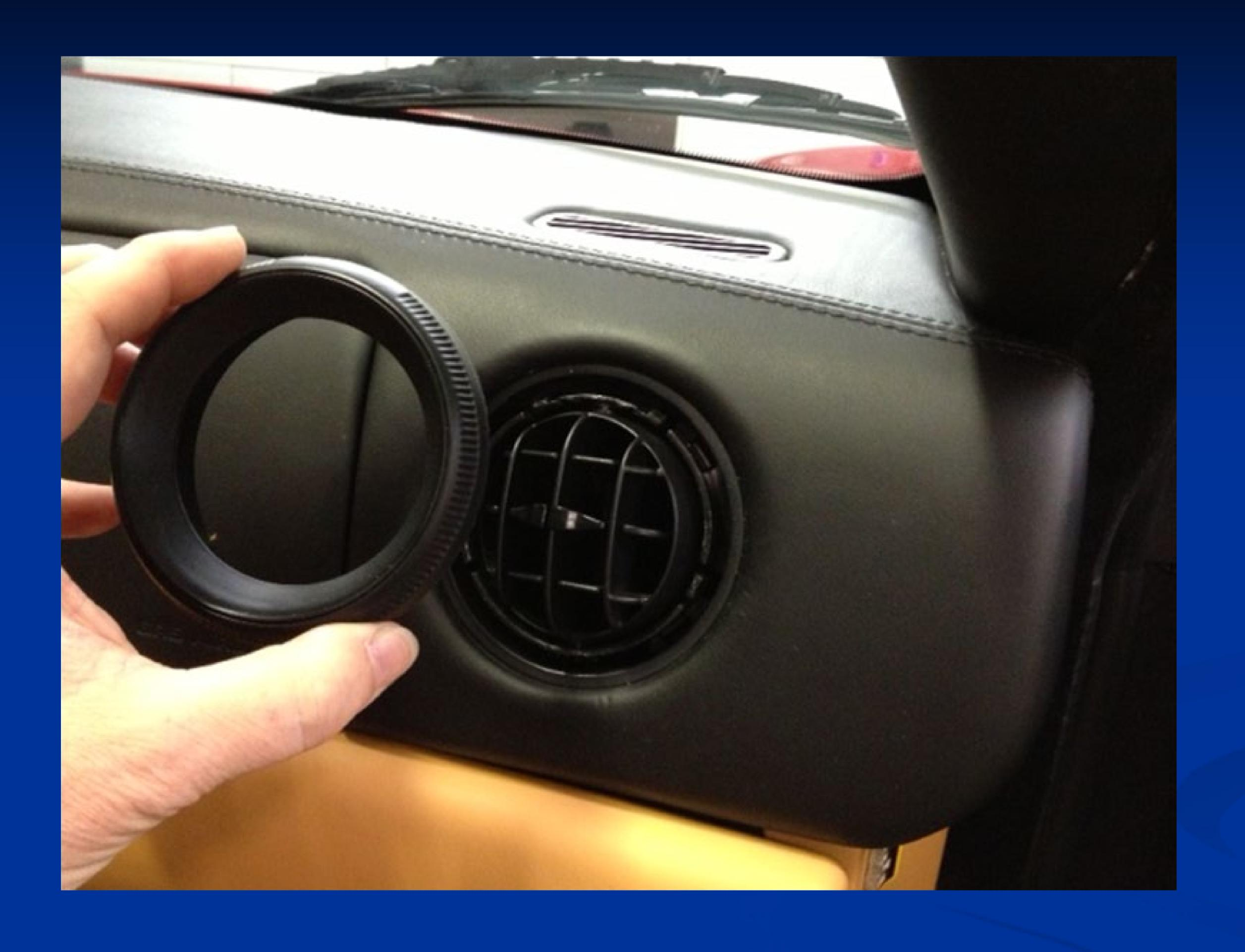
Repeat these above steps for all your vents, place them in a large gallon size Ziploc bag and send them out to us for refinishing. The last pic below I rotated the ring sideways to show you the teeth (towards the bottom of the ring) that need to be lined back up properly for the vent to open and close correctly once you re-install it. If you have any questions please do not hesitate to email and call us.
