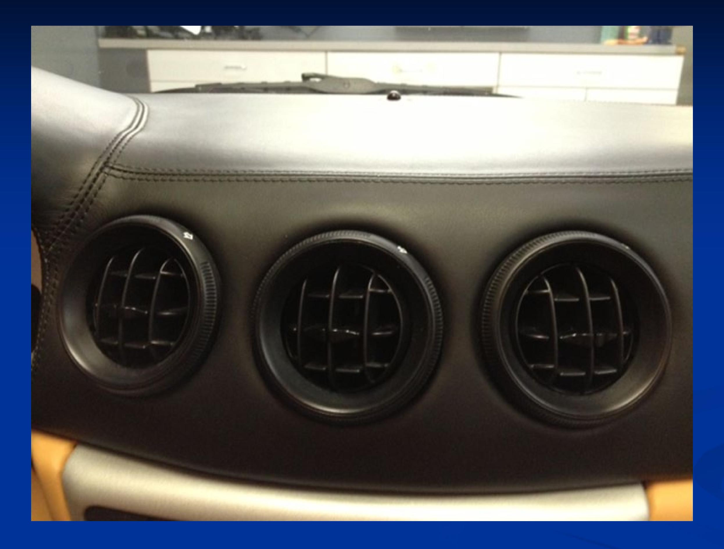
It is difficult to see, but just inside where the leather meets the ring there is a gap in the vent. This gap is where you will need to insert the screwdriver carefully. You may want to use a towel or cloth to put under the screwdriver when you begin to pry, so you don't risk damaging the leather.
