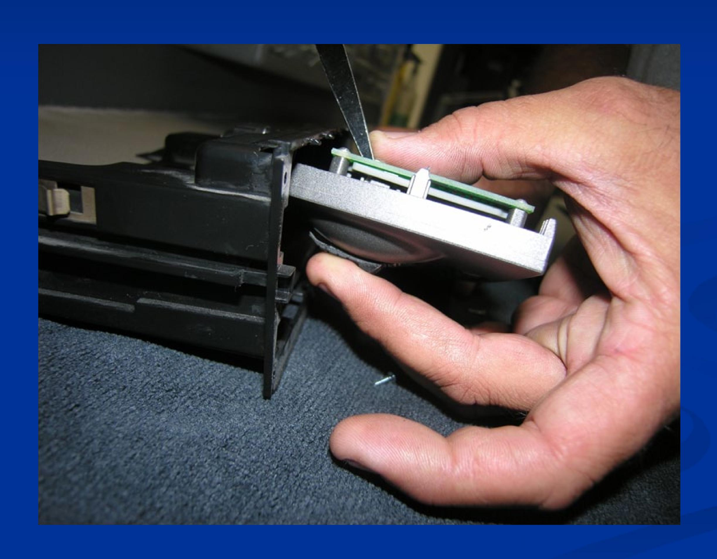
So you are pushing the white tips with your finger toward the front of the panel as you are rotating the front of the switch up and then down. The switch at this point should start to pop out.
