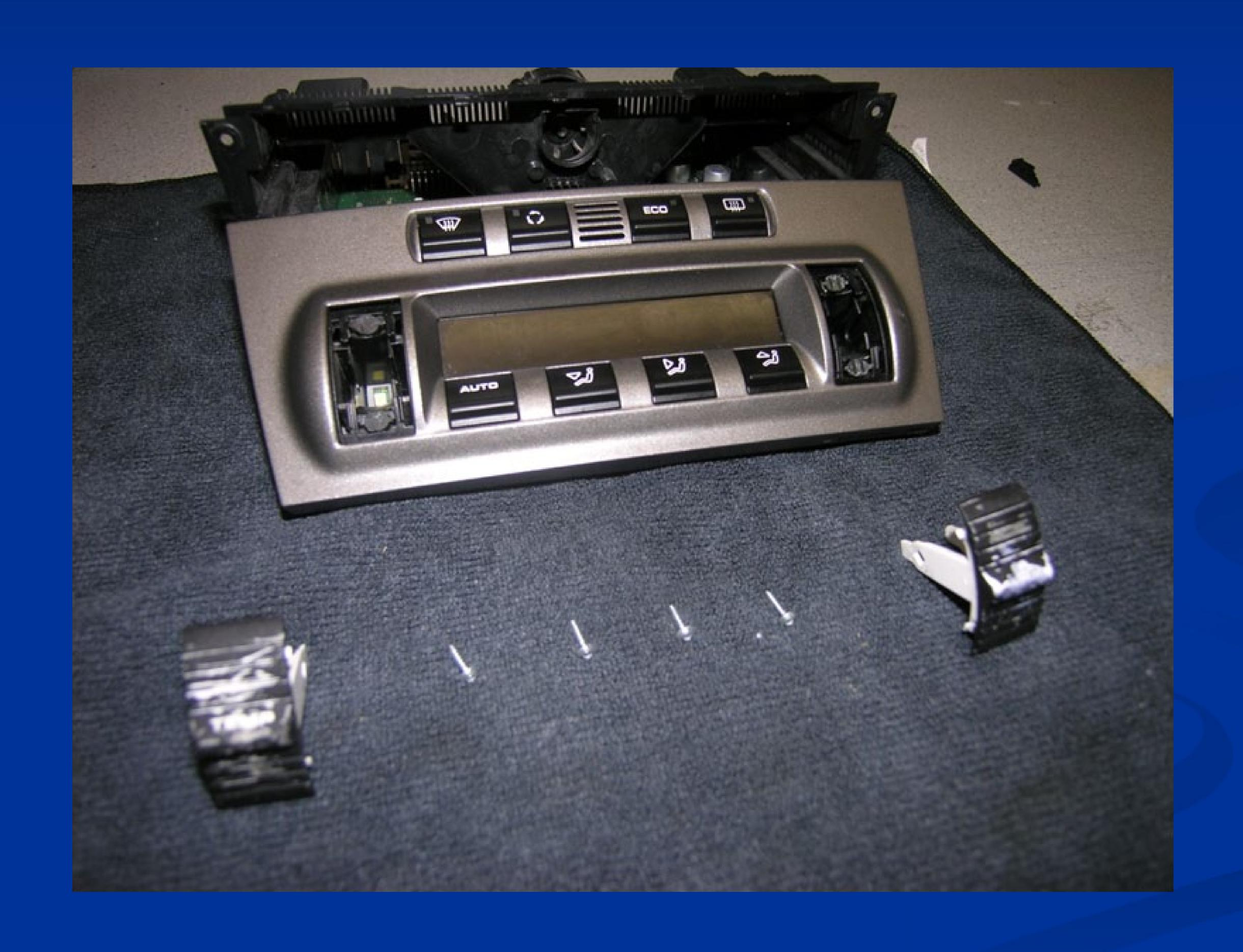
Next you are going to snap the refinished switches back into the panel. The switches are a bit too long to snap straight into place, they must go in one end at a time and rotated up and down. Push the switch into place and get it lined up.
