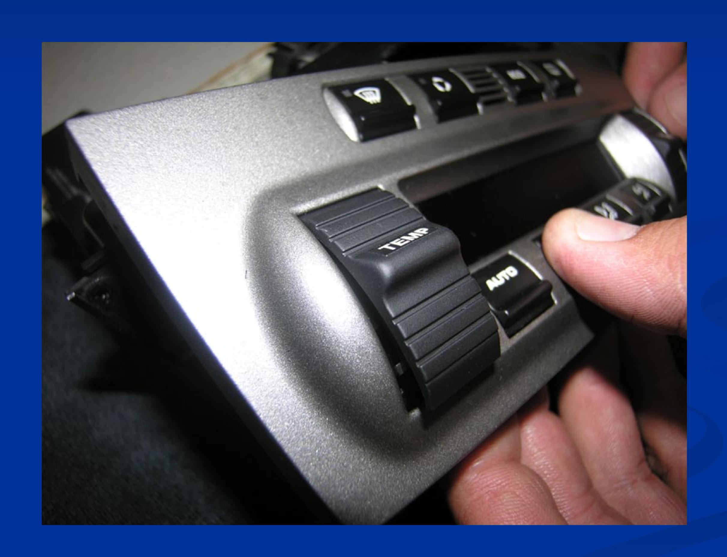
Next push the top of the switch into the panel and rotate up. The very top of the switch will actually rotate up into the panel. This will allow you room to push the bottom down and rotate that end into the panel.
