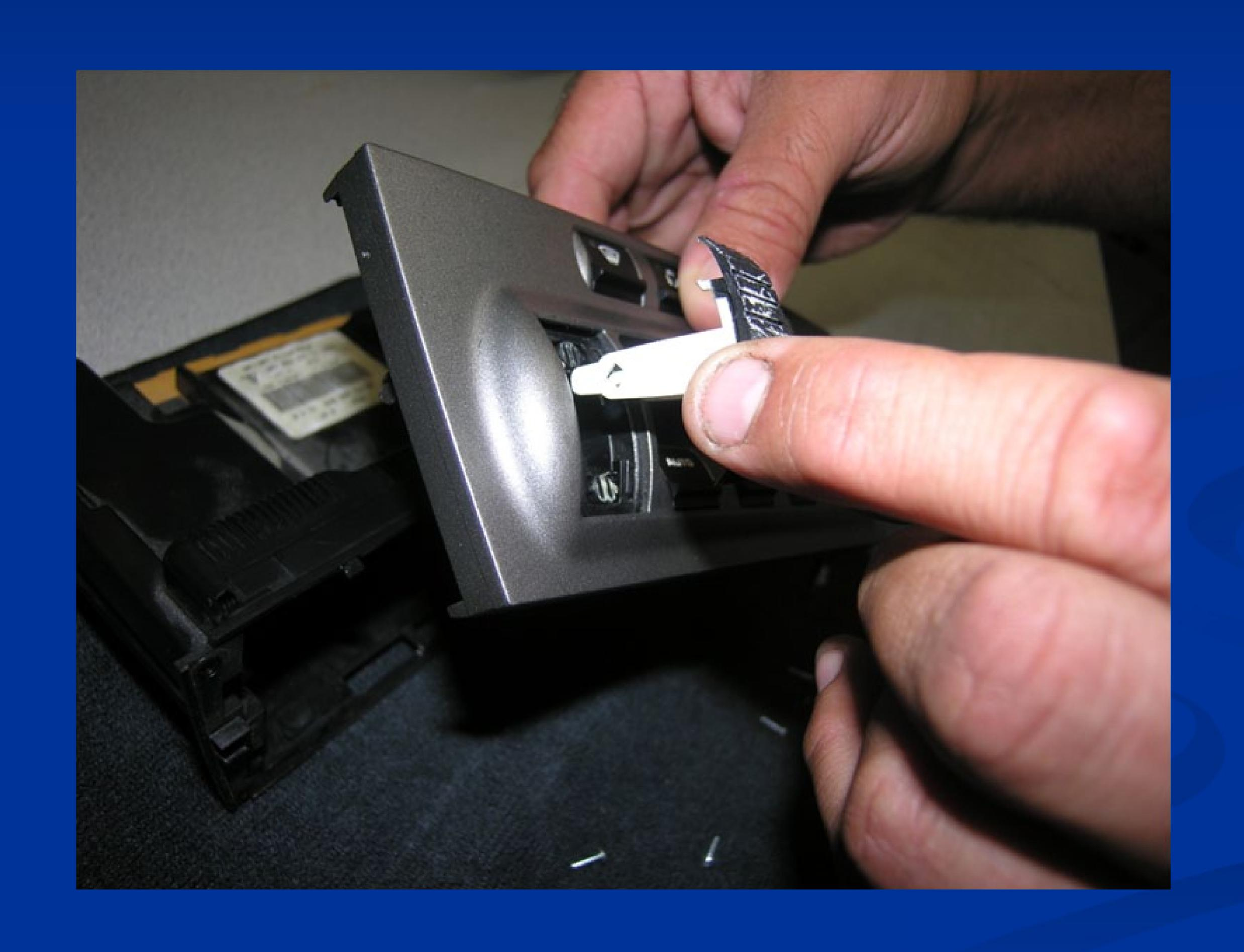
The next pic shows me grabbing one of the black sleeves inside the panel, when you push the switch, the sleeves push the electrical contact to operate the panel. The reason I am showing these sleeves is because they will fall out if you rotate the panel over or too far forward. If they fall out just put them back into the hole.
