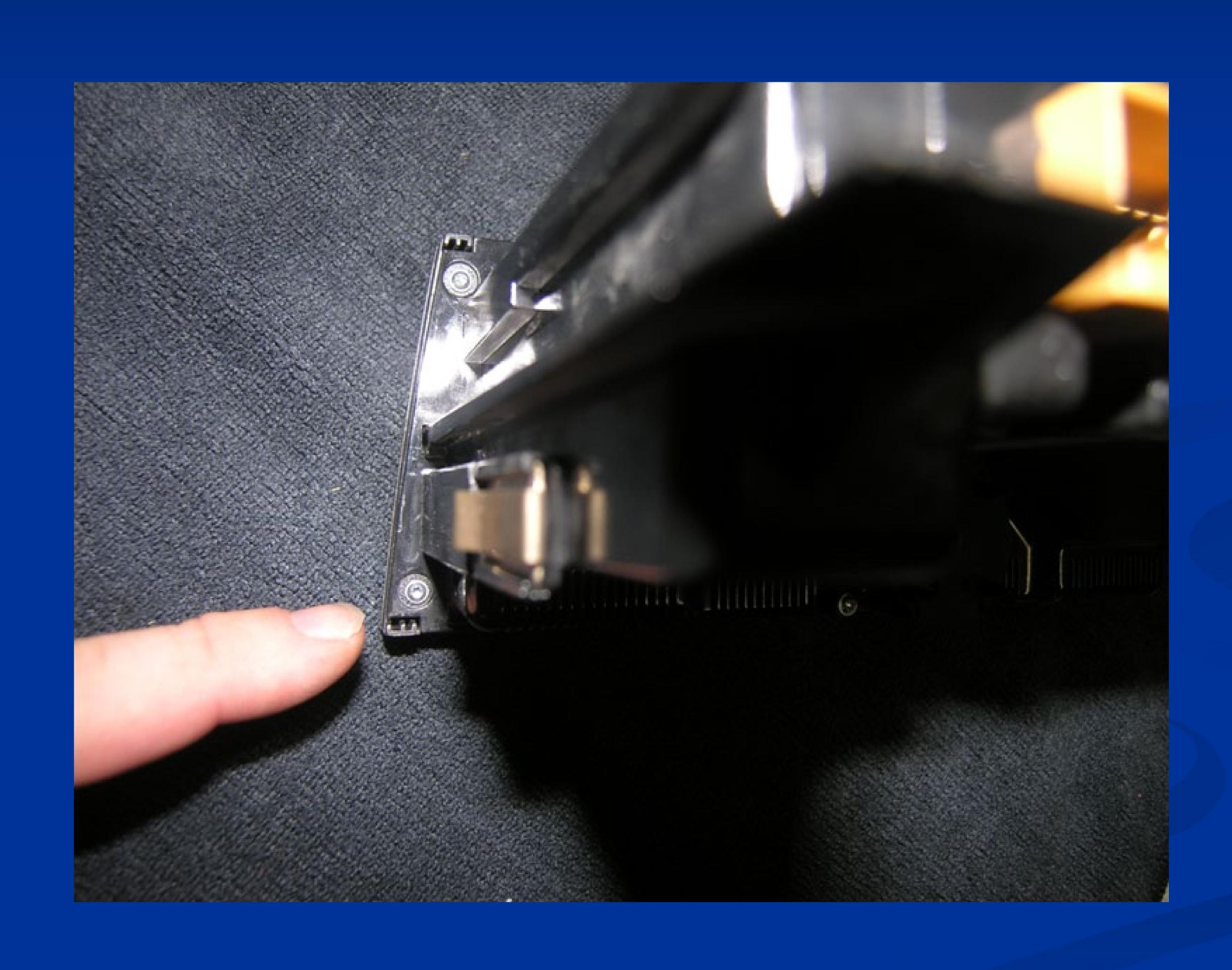
Gently pry the front panel face from the housing and lay flat
