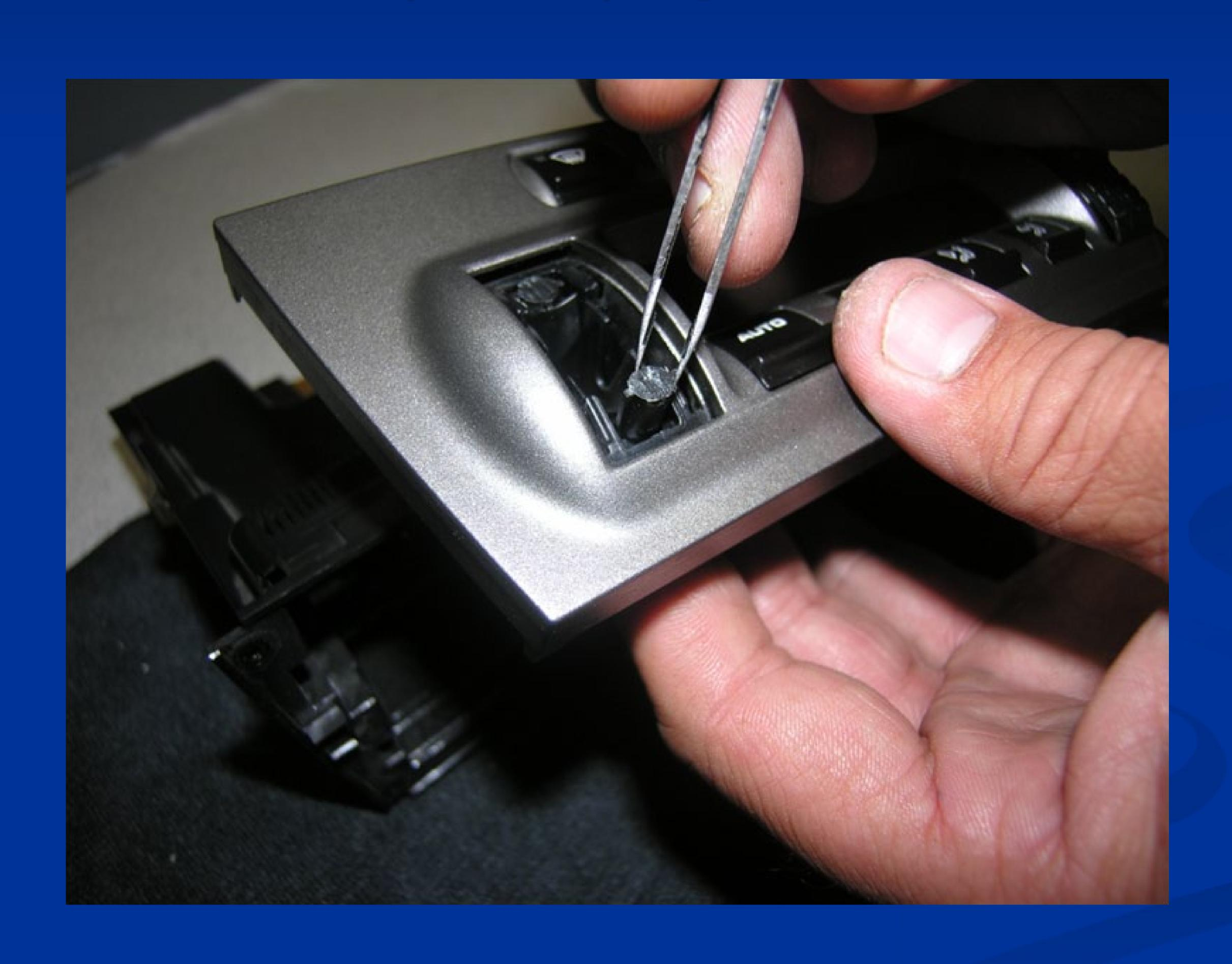
■ When your panel is disassembled you should have four screws and two switches apart.
