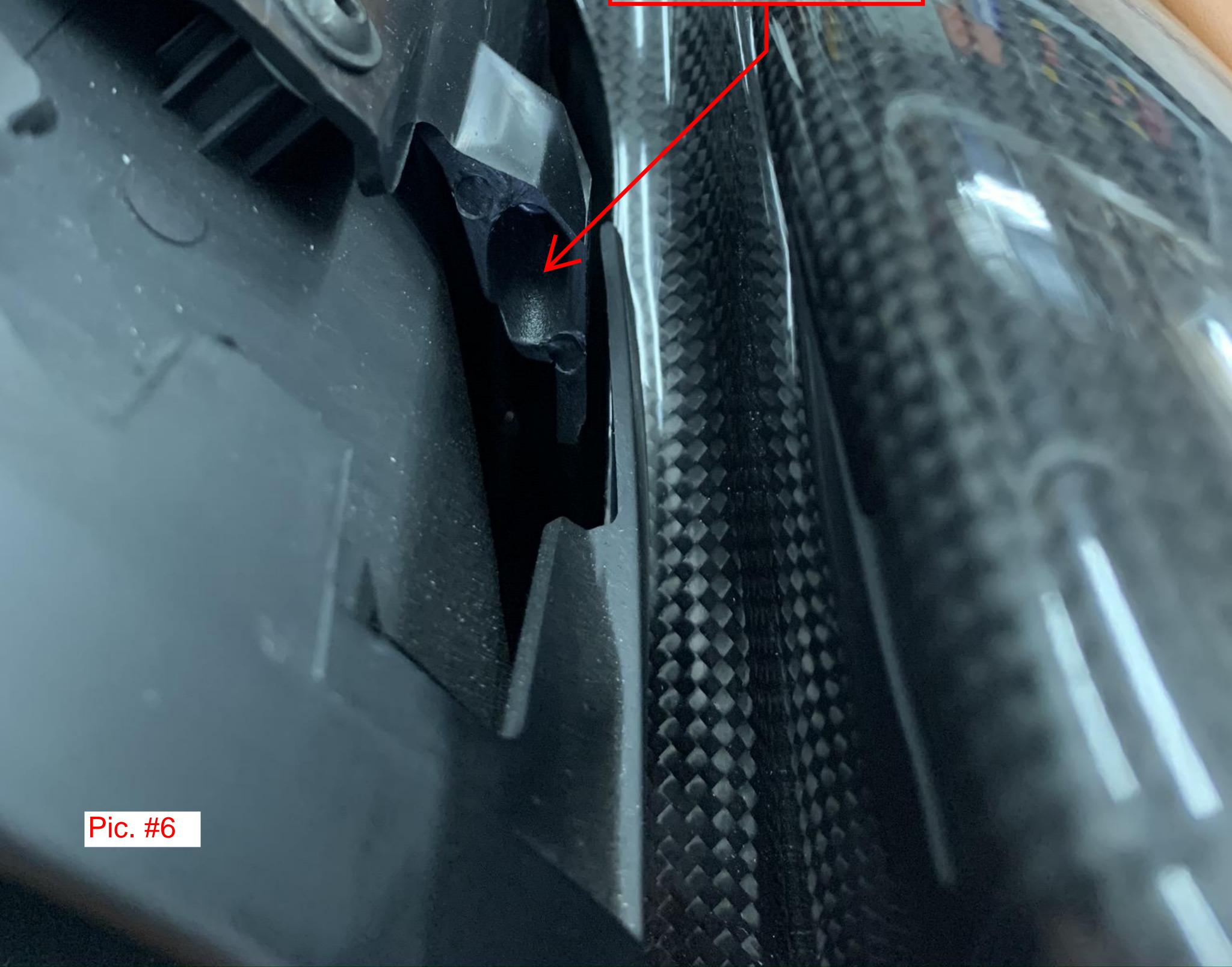
Pin 2 Goes here. It is alignment and does not snap in
