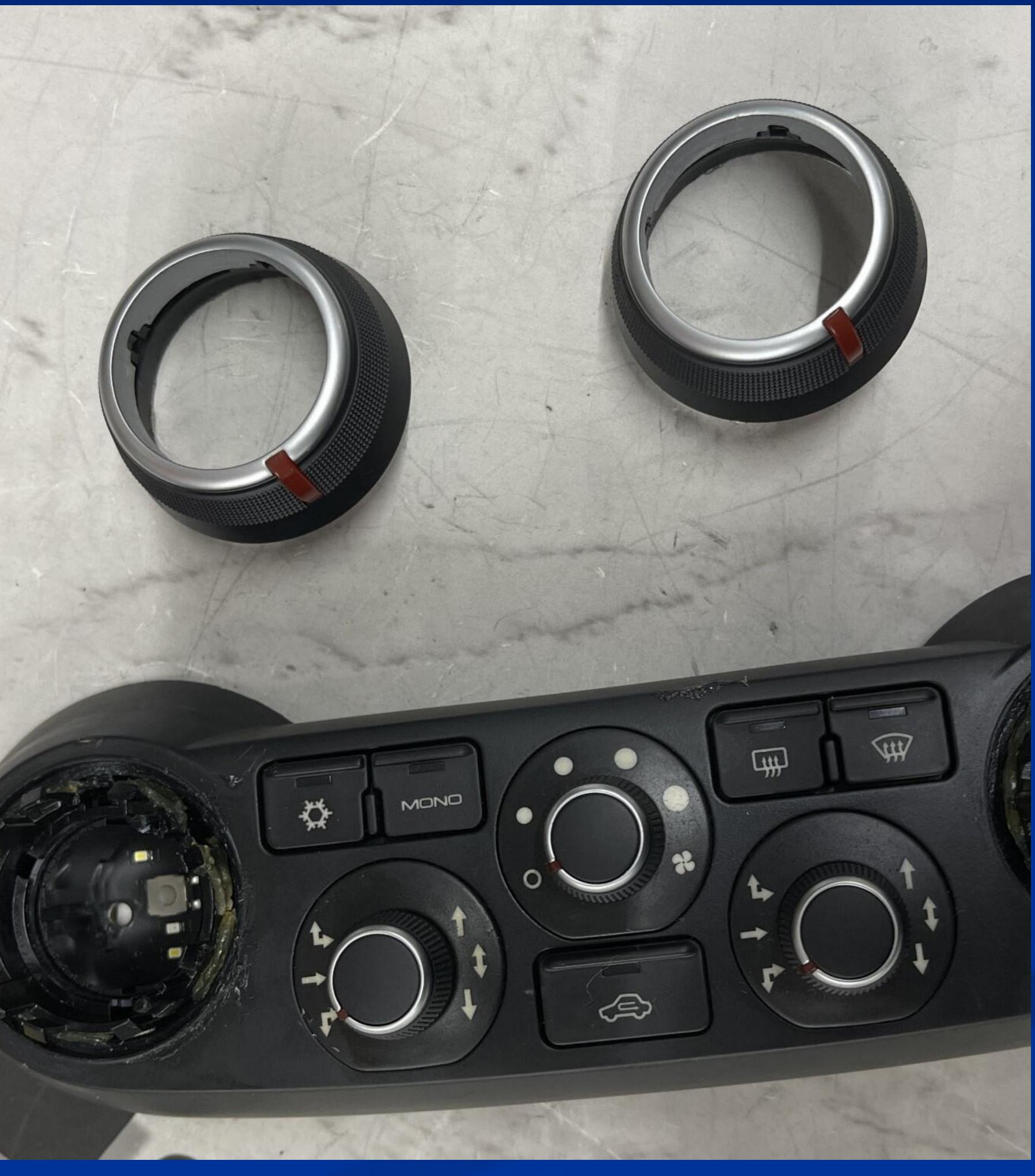
At this point, you should be able to very carefully pull out the electronics board
