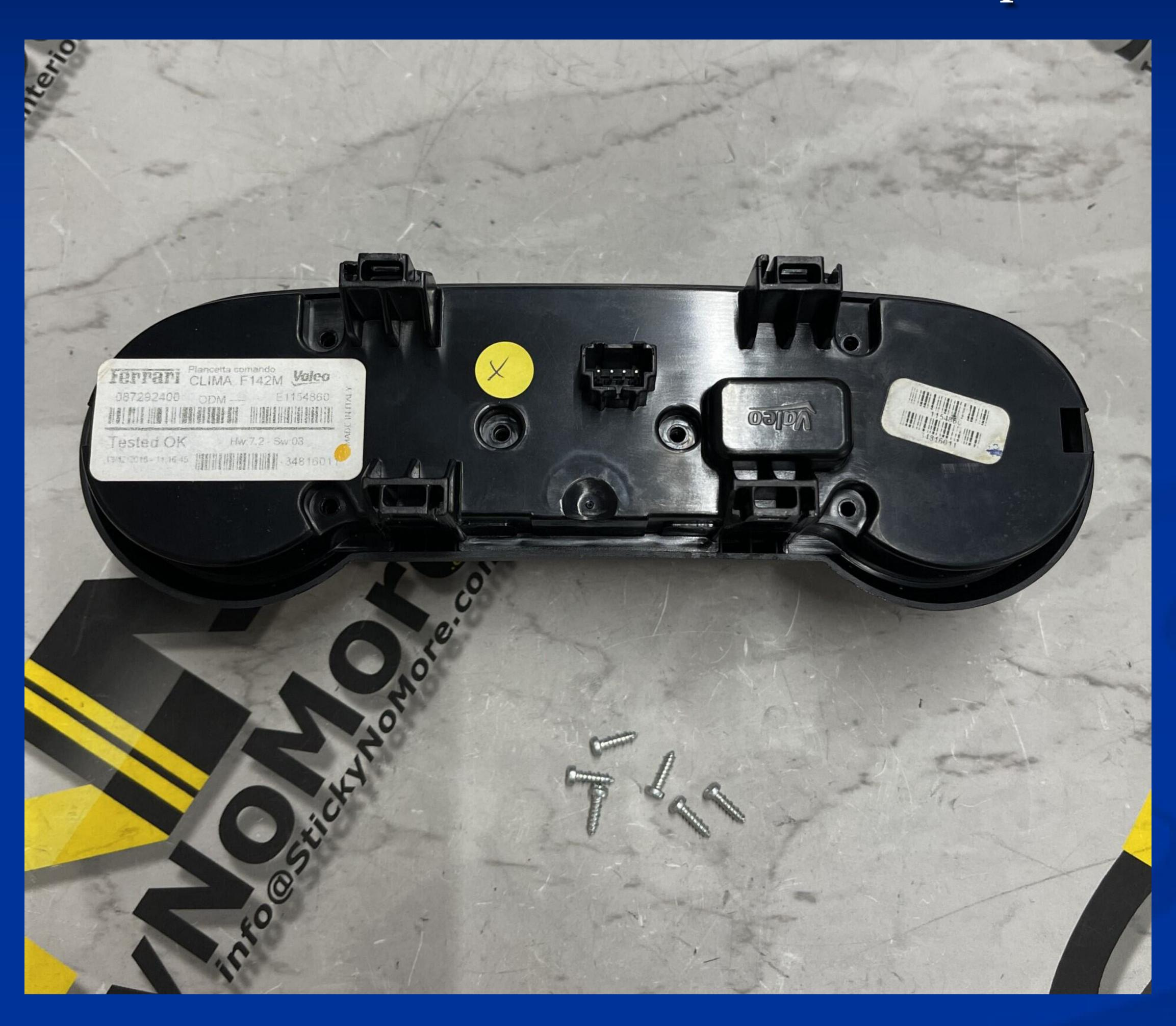
Pop the two tabs on the backside with a flat screwdriver
