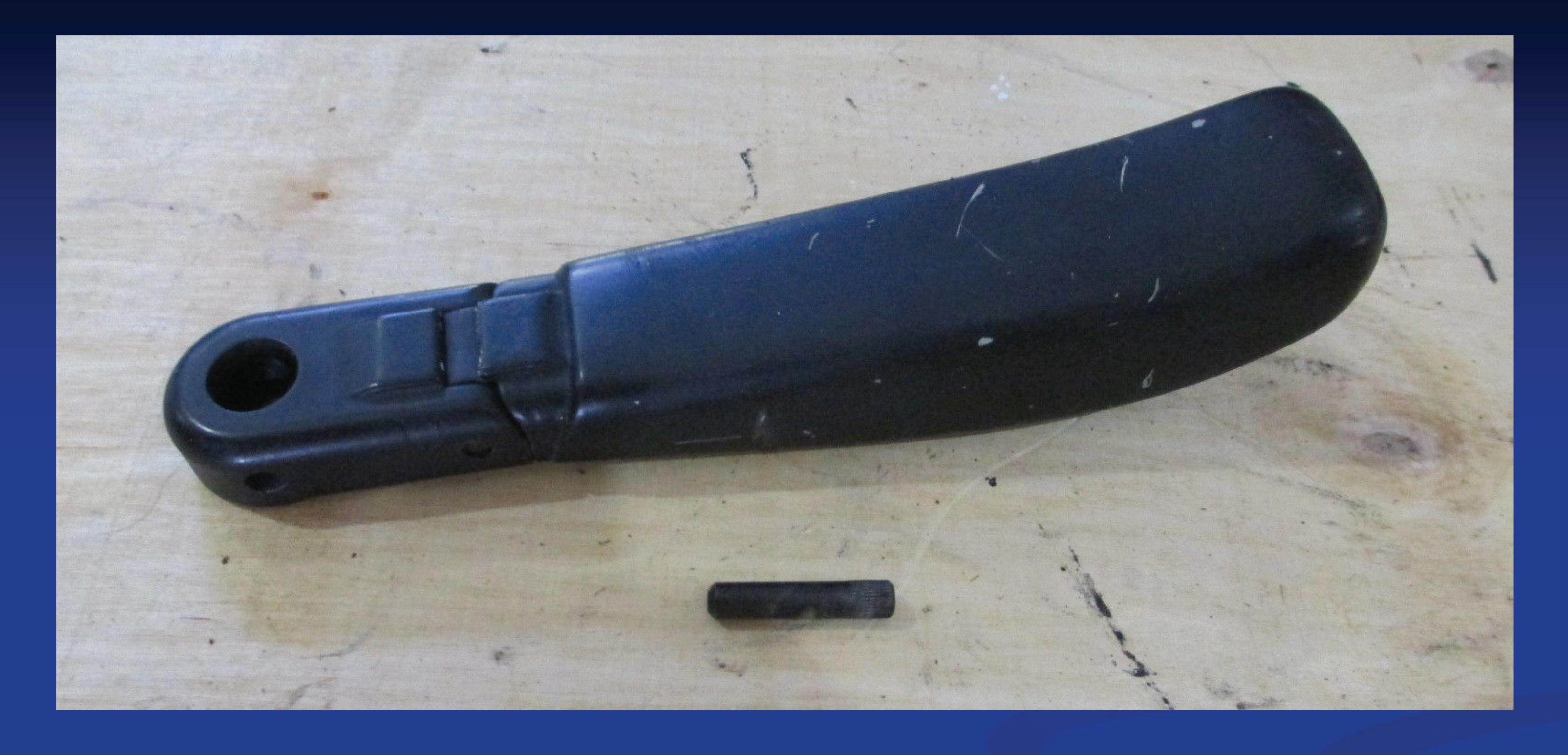
With the pin removed, gently pry the handle off the shaft with a screwdriver. Use caution to avoid getting sticky residue from the handle on the interior of the car.
