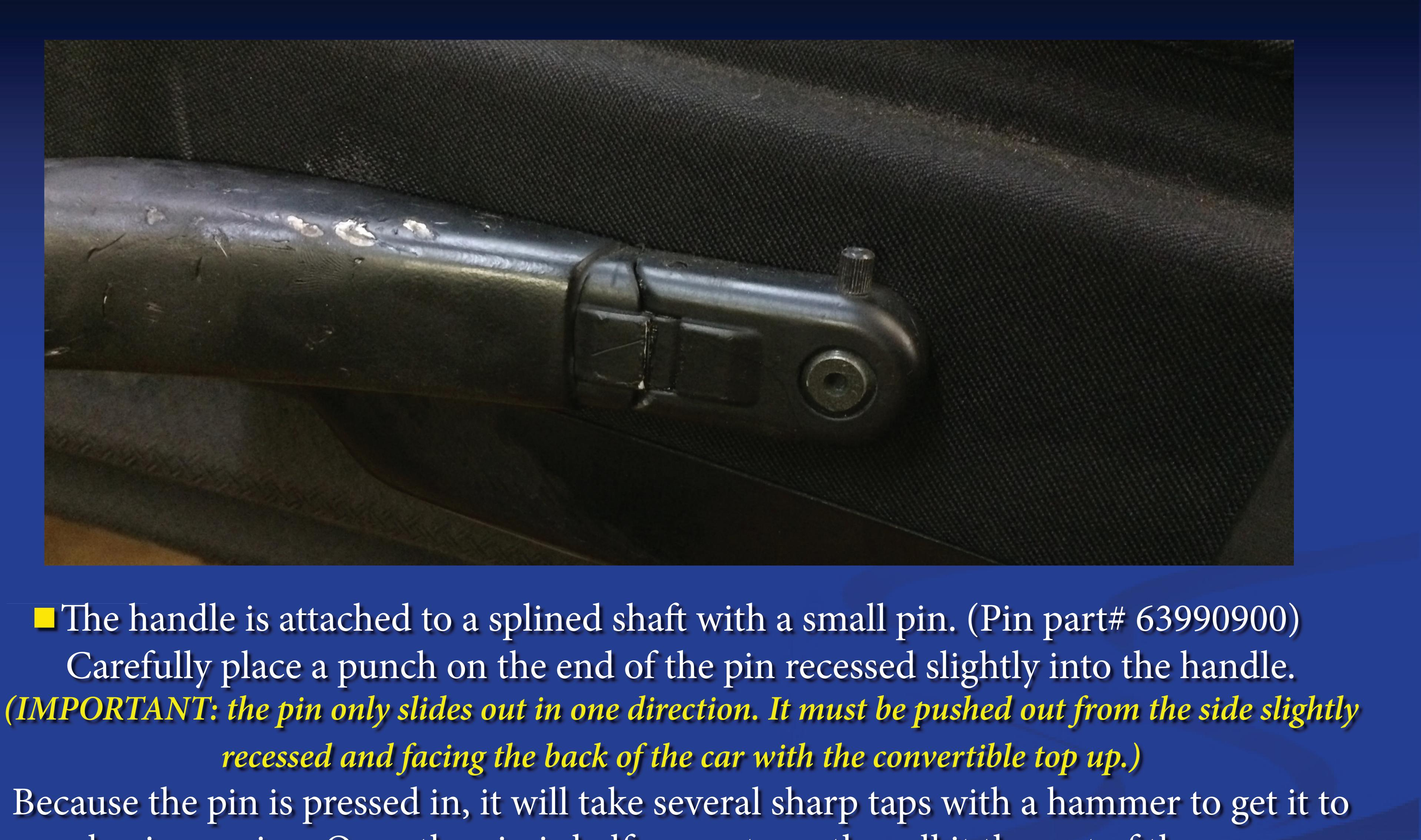
begin moving. Once the pin is halfway out, gently pull it the rest of the way.
