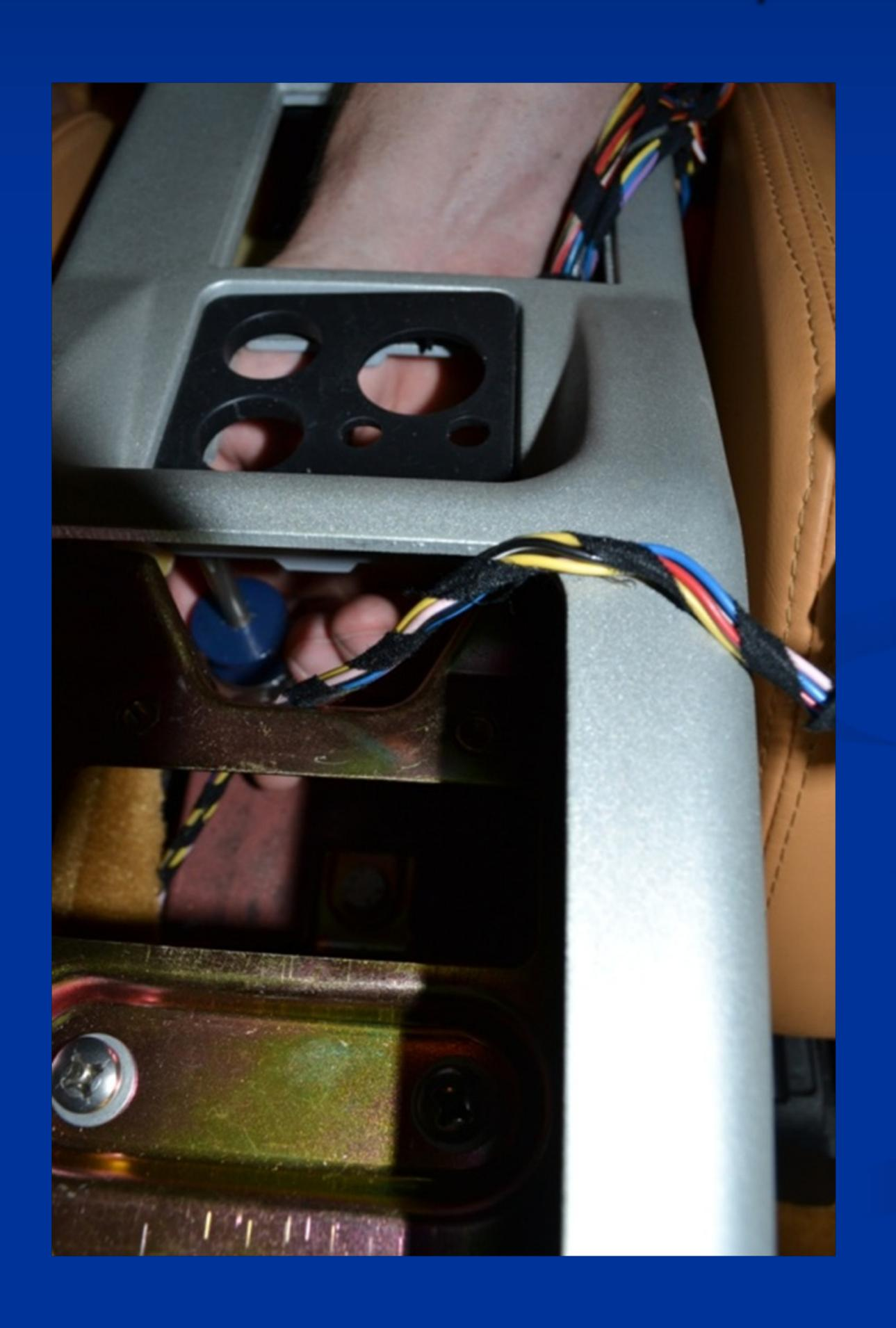
Once you have removed the four screws the trim should lift out into your hand.
