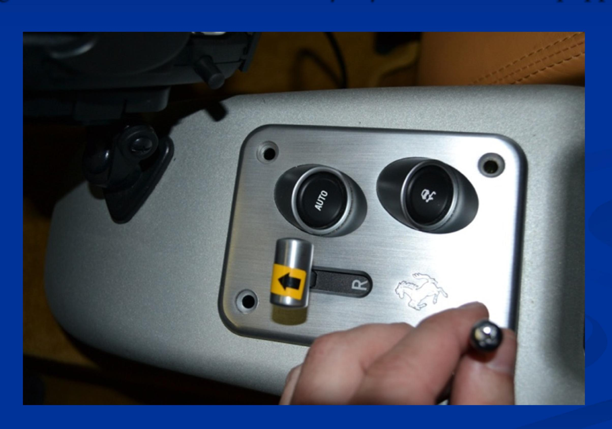
Carefully lift it out and set it out of your way. Next reach your hand into the opening where the ashtray was and unclip the three power wires to the switch and buttons.
