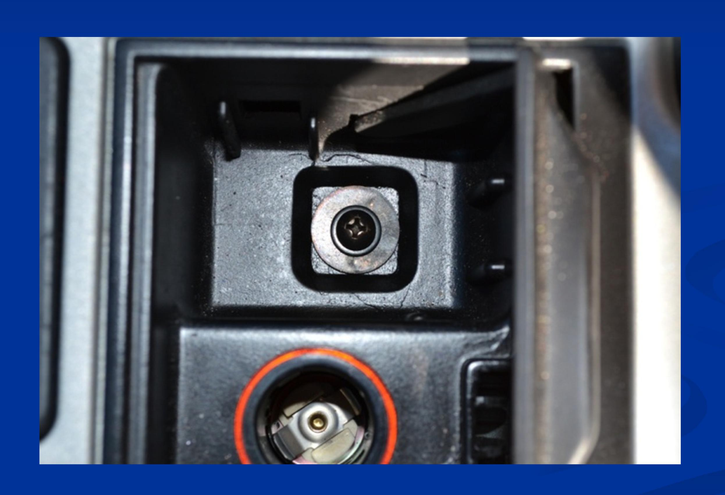
Remove the screw and lift out the ashtray assembly, unclip the power wire to the cigarette lighter, set the ashtray aside out of your way. Next remove the four screws holding the T reserve handle assembly if you have an F1 equipped car.
