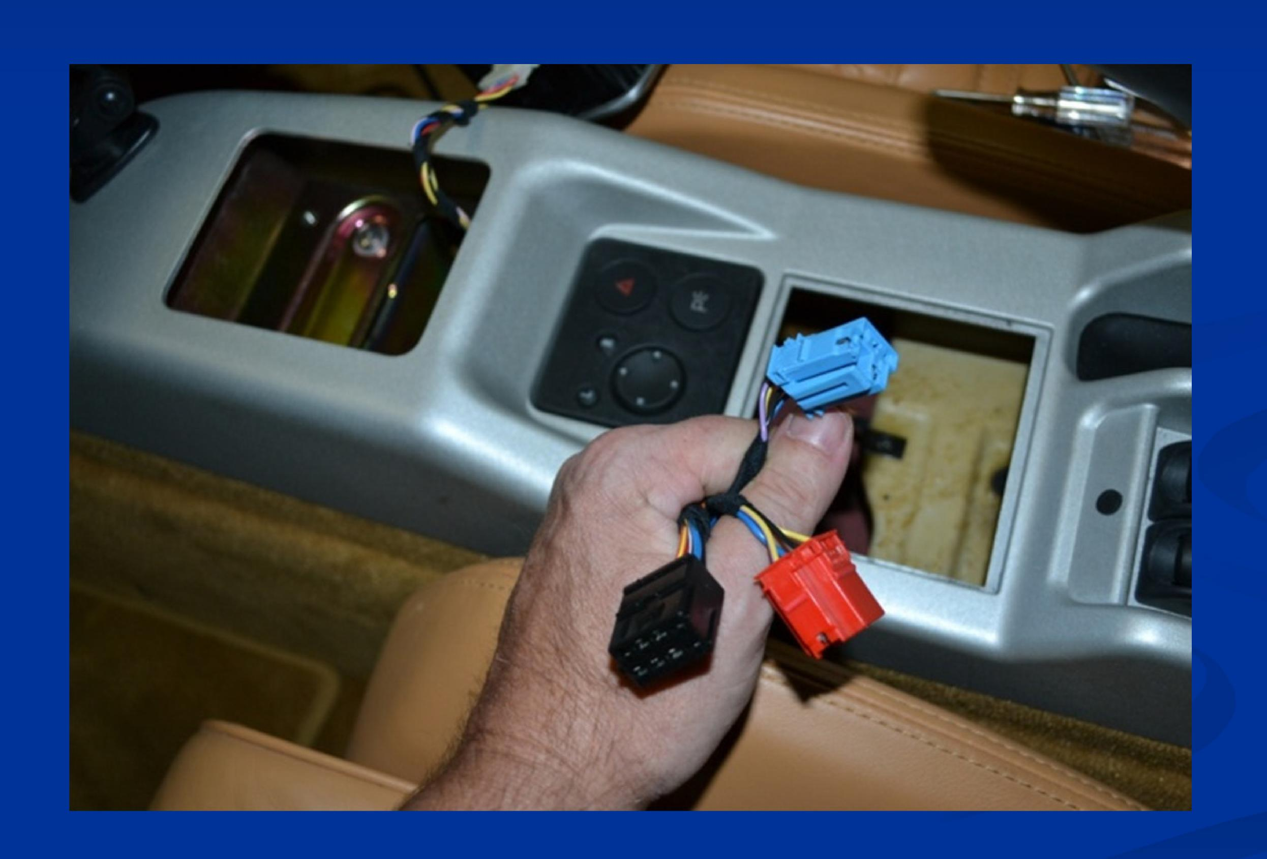
■ You're going to need a small Phillips screwdriver. There are four screws, one at each corner under the trim holding it into place. You can reach into the opening and feel the four screw heads. They are NOT easy to remove because there is not a lot of work space in the opening, but with patience and a small hand you will get them out.
